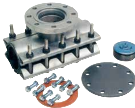
TEAM's FloStop II heavy-duty Line Stop fittings are available in sizes 4" (ND 100mm) to 12" (ND 300mm). 4" (ND 100mm), 6" (ND 150mm), and 8" (ND 200mm) fittings are stainless steel. 10" (ND 250mm) and 12" (ND 300mm) are carbon steel.
